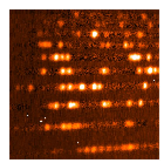
Water vapor as seen in 30 cm of lab air at Ball. Many lines are saturated and/or pressure broadened.
